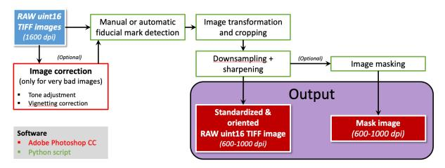
**Figure 12.** Image pre-processing workflow developed at the RMCA for the preparation of the historical aerial photographs for the photogrammetric processing.
