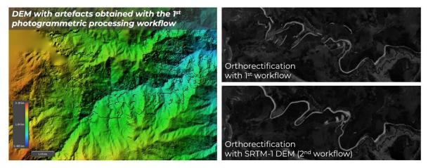
**Figure 15.** Comparison of the two photogrammetric workflows for low quality datasets, in mountainous environment. The left frame shows artefacts in a DEM derived from the aerial photographs, when image overlapping is insufficient. The frames on the right show how bad topographic reconstruction can lead to errors in the orthomosaic (top-right image), while an external DEM can solve most of these errors when it is used for orthorectification.
