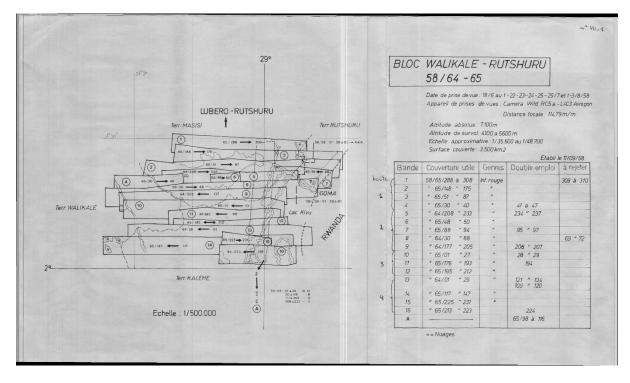
Figure 10. Example of a flight plan for the acquisition of historical aerial photographs.
