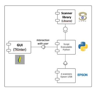
**Figure 11.** Mass-scanning infrastructure of the RMCA. Four flatbed photo scanners (photo on the left) digitise the historical aerial photographs in parallel, using the SANE library and a Python script (scheme on the right).
